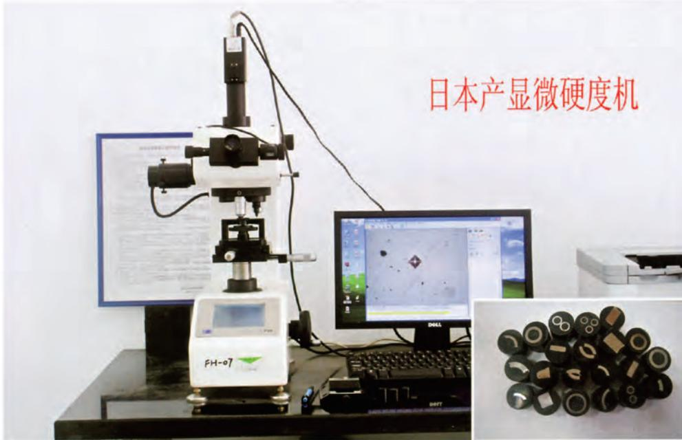
日本产显微硬度机 Japan made microhardness instrument
