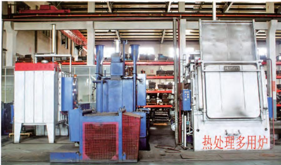
热处理多用炉 Multi-purpose furnace
