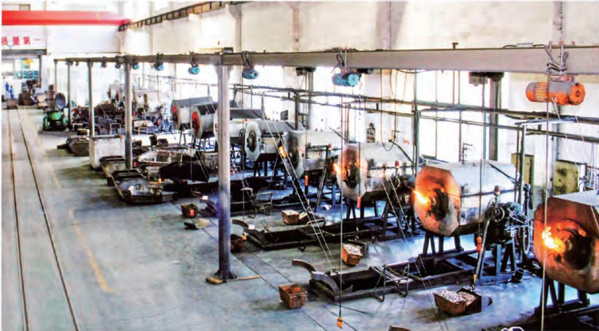
滚筒式渗碳炉 Rolling type case hardening furnace
