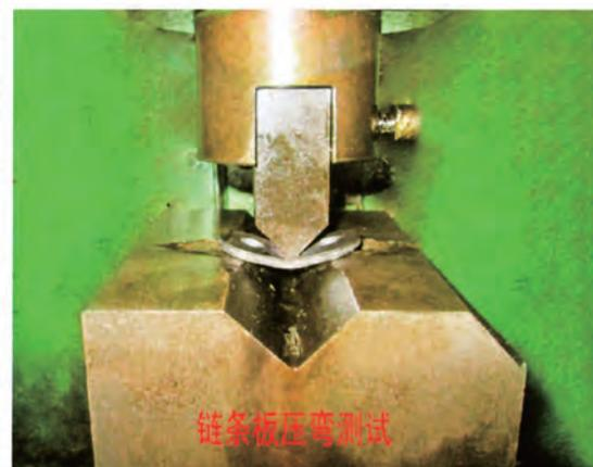
链条板压弯测试 Plate bending tester
