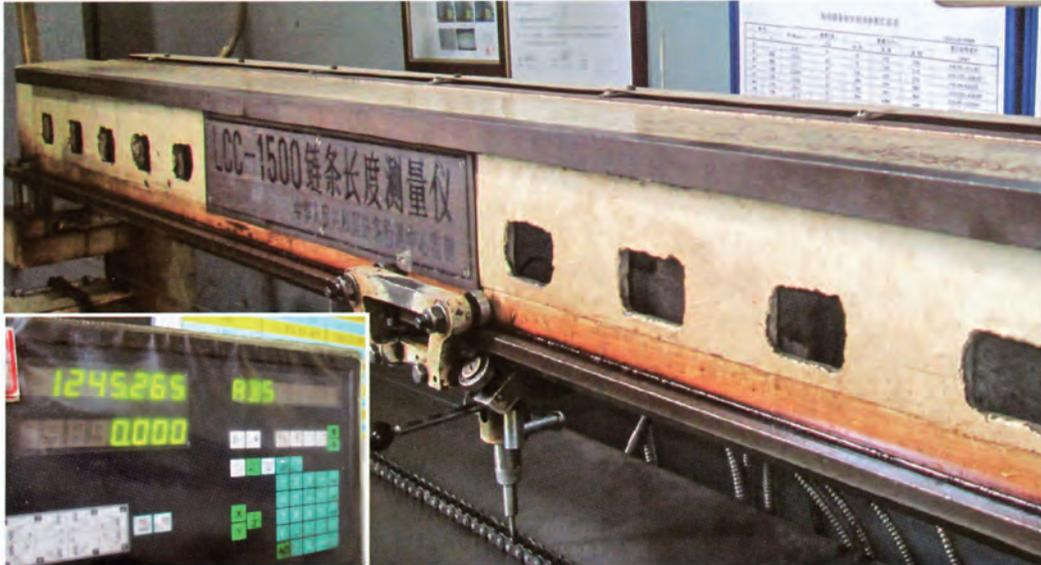
长度精度测量 Length accuracy measuring machine
