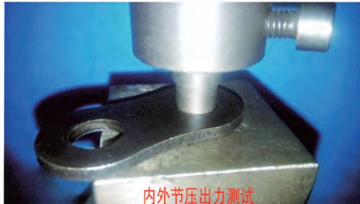
内外节压出力测试 Push out force tester for inner link and outer link
