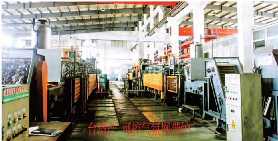
台湾产 可控气氛网带炉 Taiwan made atmosphere controlled mesh belt furnace
