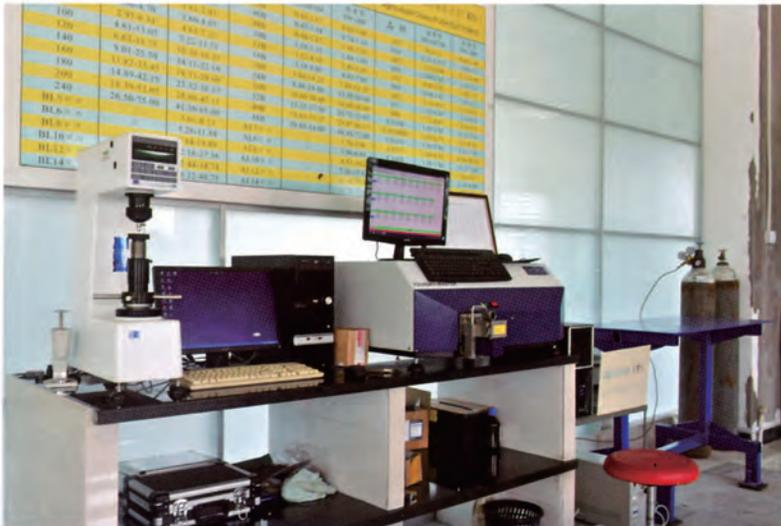
德国产材料分析光谱仪 Germany made material spectrum analyzer
